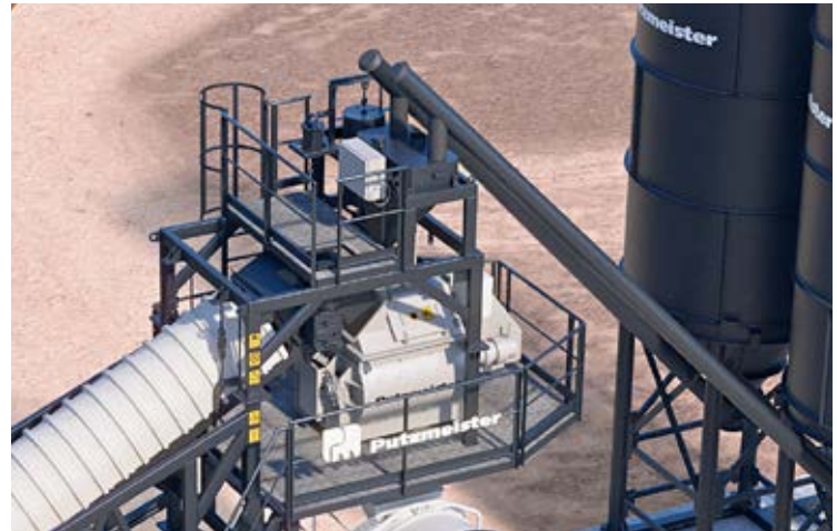
#2 Second Level Surround Platform for easy accessibility and faster maintenance
